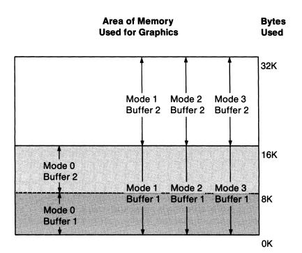
In a 128K Apple III, the entire 32K display buffer space shown is available for graphics. For any given graphics mode, the two display buffers occupy separate areas of memory, so that you can switch back and forth between their independent images. Also, both of the mode 0 display buffers occupy separate areas of memory from display buffer 2 of any other mode. This means you can switch between independent images in mode 0's buffer 2, for example, and mode 3's buffer 2.
